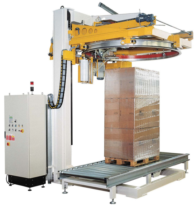
Fig. 2 Example of automatic machine for stretch-wrapping pallets
